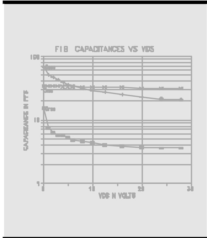
Fig 6. Capacitance vs Vds for Polyfet F1B devices
