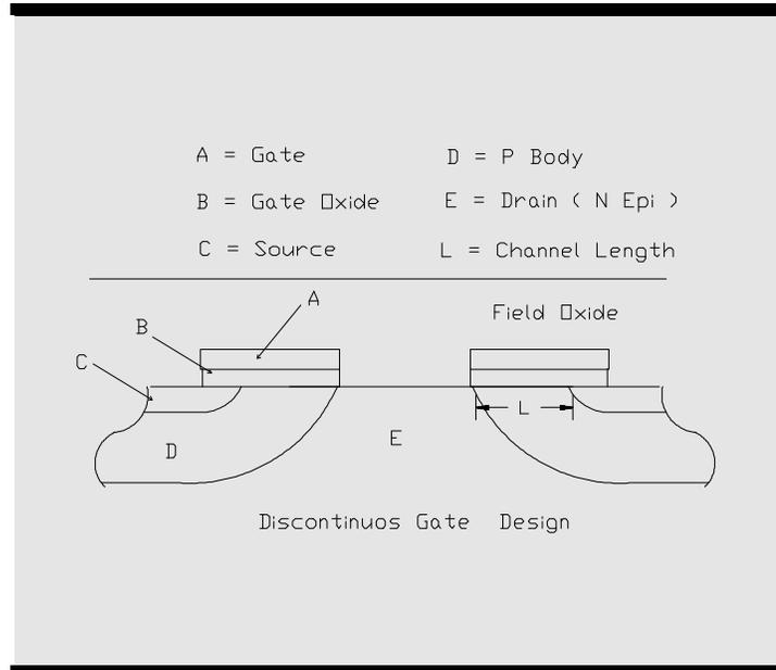
Fig 1. Cross Section of Vertical DMOS transistor
