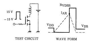
$$\begin{array}{l} T_{ch} = 25^{\circ}C \; (Initial) \\ Peak \; I_{AR} = 5 \; A, \; R_G = 25 \; \Omega \quad E_{AS} = \frac{1}{2} \cdot L \cdot I^2 \cdot \; (\frac{BVDSS}{BVDSS - V_{DD}}) \\ V_{DD} = 24 \; V, \; L = 1.0 \; mH \end{array}$$
