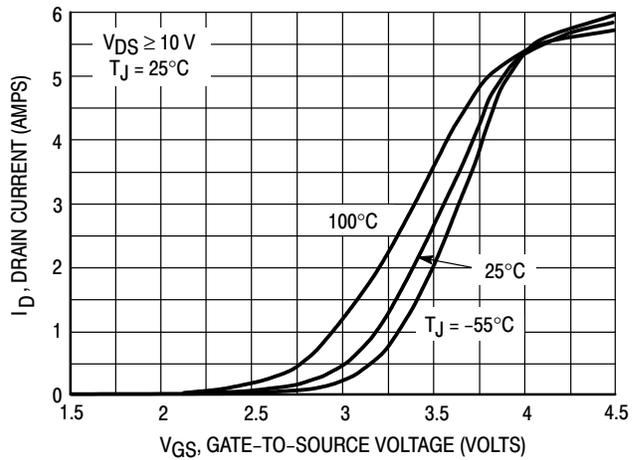
Figure 2. Transfer Characteristics
