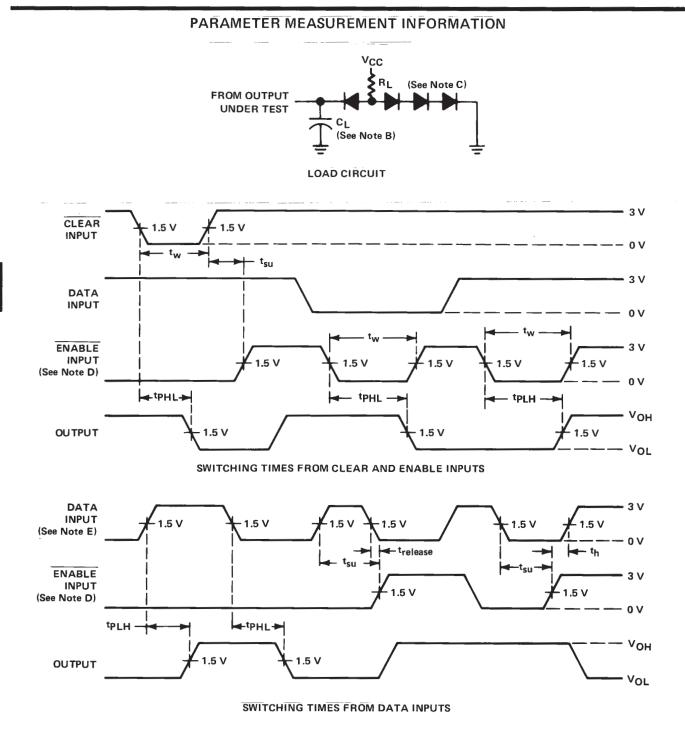
NOTES: A. Input pulses are supplied by generators having the following characteristics:  $t_r \le 10$  ns,  $t_f \le 10$  ns, PRR = 1 MHz, duty cycle  $\le 50\%$ ,  $Z_{out} \approx 50\Omega$ .
