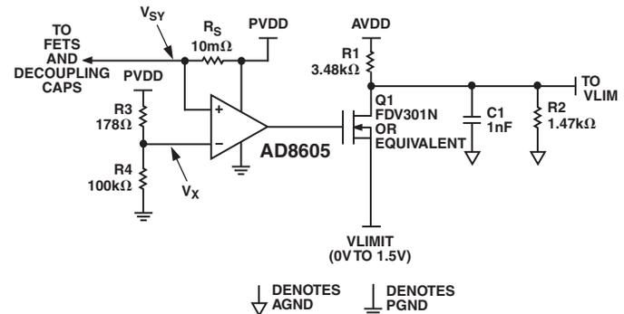
Figure 21. Setting a Maximum Output Current Limit
