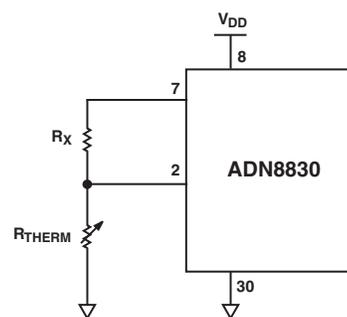
Figure 3. Connecting a Thermistor to the ADN8830
