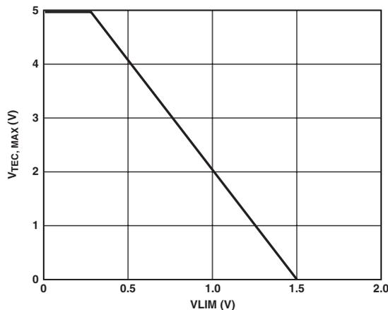
Figure 12. VLIM Voltage vs. Maximum TEC Voltage
