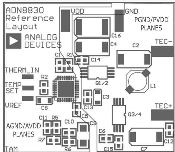
Figure 19. Top Layer Reference Layout for ADN8830
