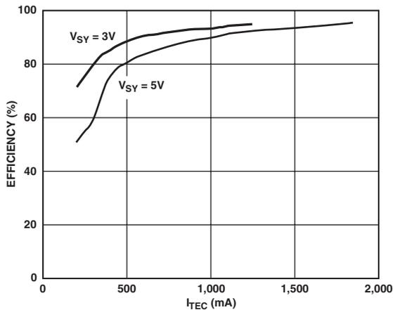
Figure 17. Efficiency with  $f_{CLK} = 200\text{ kHz}$
