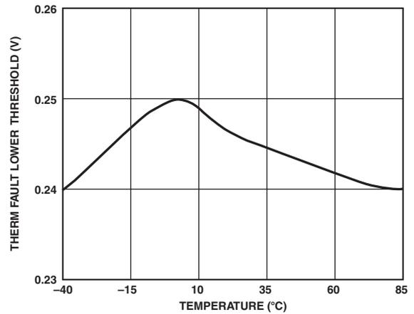
TPC 12. Short Thermistor Fault Threshold vs. Temperature
