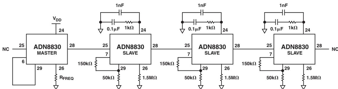
Figure 8. Multiple ADN8830 Devices Using a Daisy Chain
