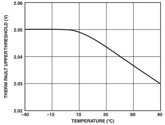
TPC 11. Open Thermistor Fault Threshold vs. Temperature
