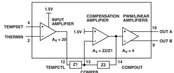
Figure 2. Signal Flow Block Diagram of the ADN8830
