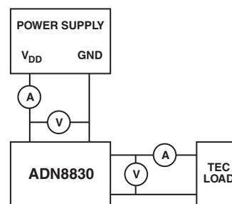
Figure 15. Measuring Efficiency of the ADN8830 Circuit
