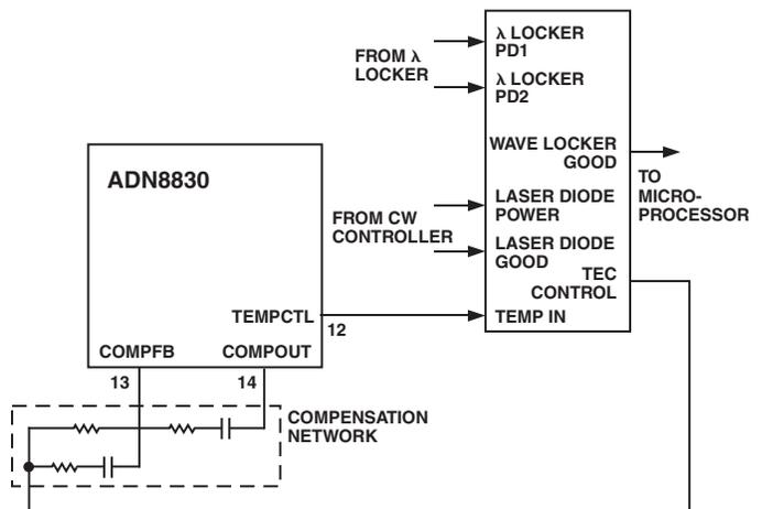
Figure 11. Using the ADN8830 with a Wave Locker
