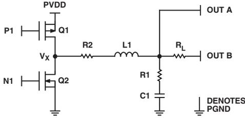
Figure 14. Equivalent Circuit for PWM Amplifier and Filter
