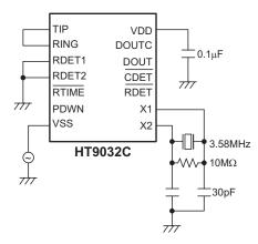
Supply current testing: All, except PDWN and RTIME, unwired pins are left floating.
