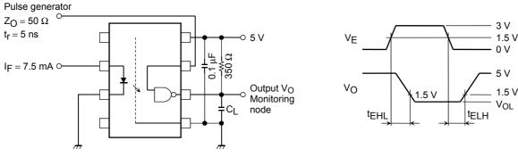
CL is approximately 15 pF which includes probe and stray wiring capacitance.
