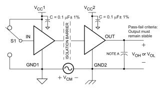
A.  $C_L = 15$  pF and includes instrumentation and fixture capacitance within  $\pm 20\%$ .
