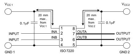
Figure 18. Typical ISO7220 Application Circuit
