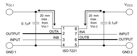
Figure 19. Typical ISO7221 Application Circuit
