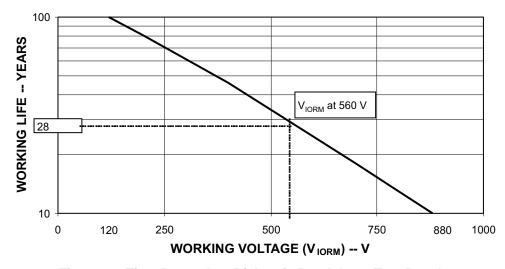
Figure 20. Time Dependent Dielectric Breakdown Test Results
