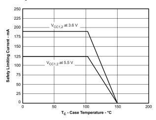
Figure 5. SOIC-8  $\theta_{\text{JC}}$  THERMAL DERATING CURVE per IEC 60747-5-2
