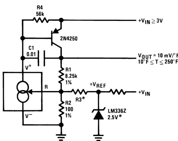
\*Select  $R_3 = V_{REF}/583\mu\text{A}$ .  $V_{REF}$  may be any stable positive voltage  $\geq 2\text{V}$ . Trim  $R_3$  to calibrate.
