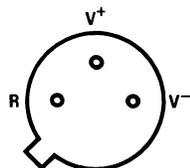
V<sup>-</sup> Pin is electrically connected to case.
