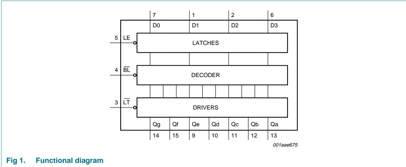
Fig 1. Functional diagram
