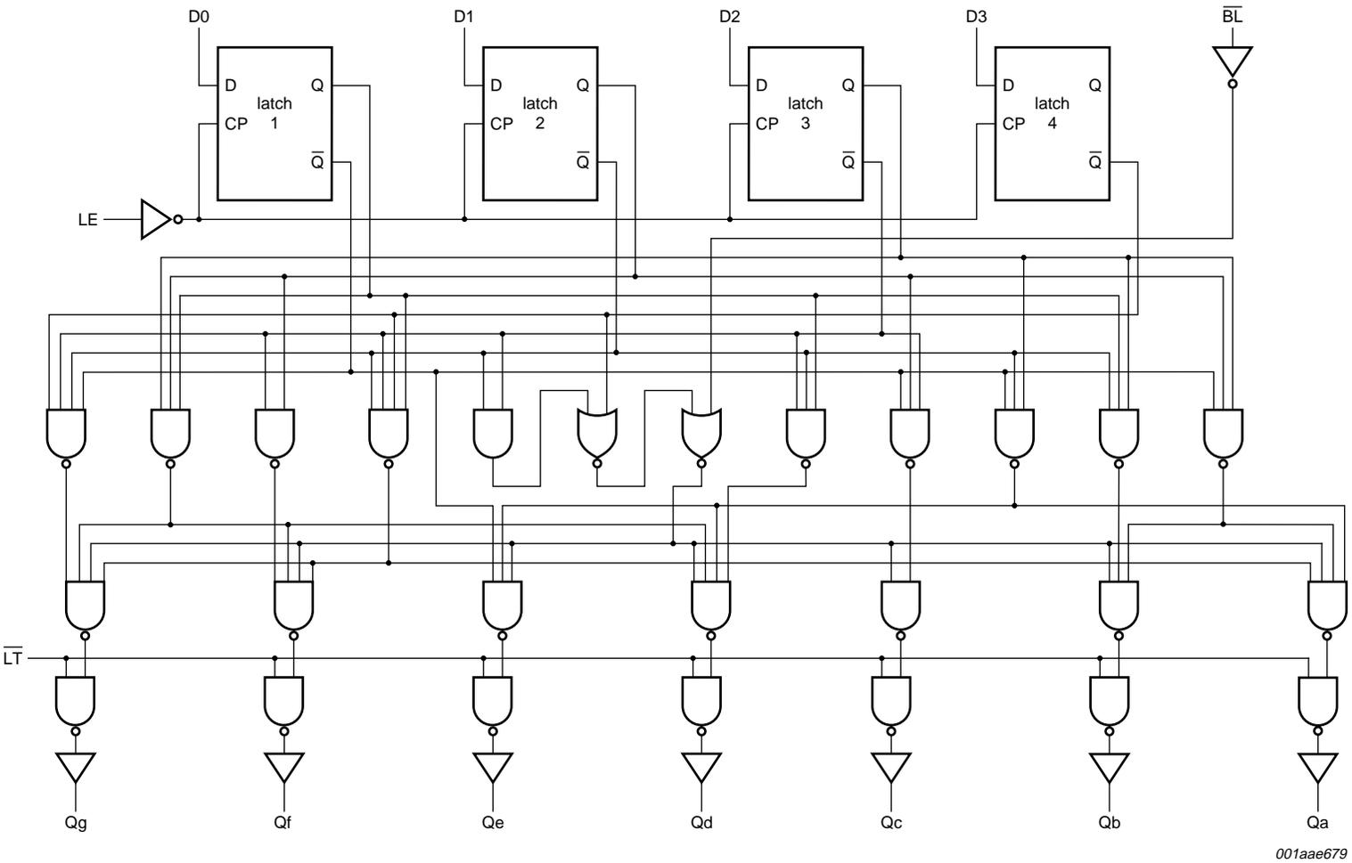
Fig 3. Logic diagram
