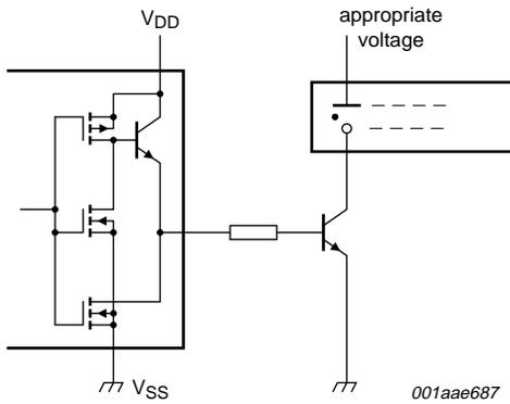
**Fig 13. Connection to gas discharge display readout**
