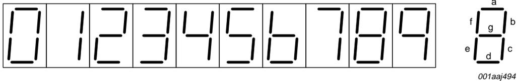
Fig 5. Seven segment digital display with segment designation
