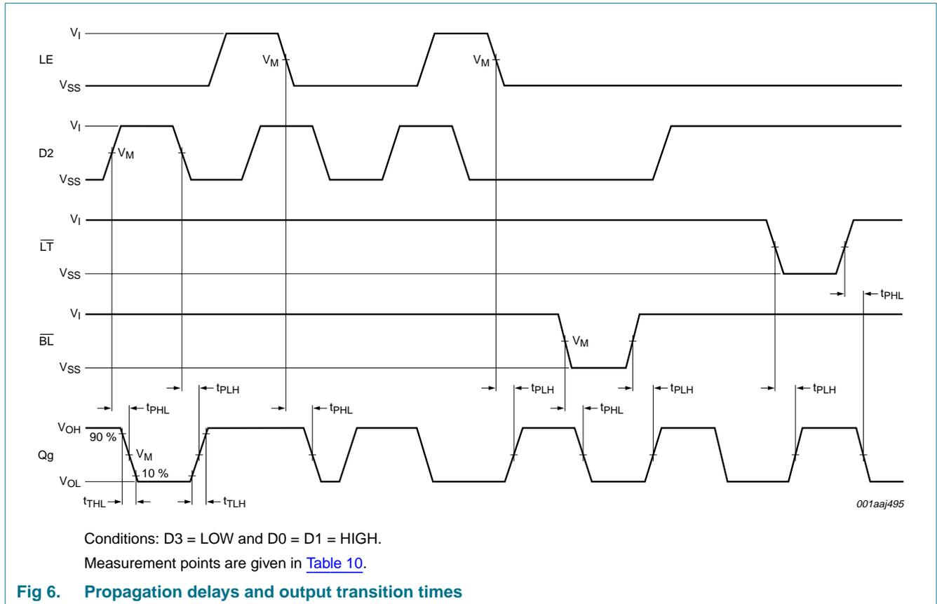
Fig 6. Propagation delays and output transition times
